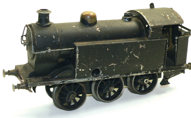
Featured item: Lot 255 Walker-Fenn O-gauge clockwork 0-6-0 Tank Locomotive. Needs some attention but a rare and unusual model with adjustable governor.
